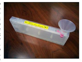
place for use the next time you need to refill. Repeat the filling process with each cartridge in turn using a clean funnel for each cartridge and ensuring you fill the correct color ink into the correct color cartridge.
