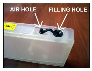
bung into the air vent hole is when you have the cartridge out of the printer, or if you intend not to use the printer for an extended period of time – putting the bung in the air vent hole will prevent ink evaporation.
