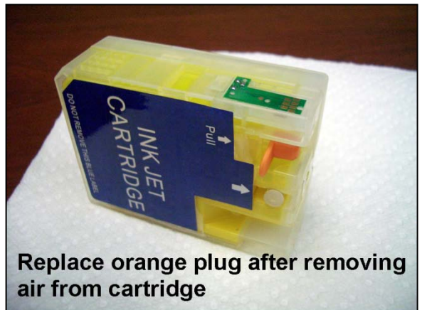
Remove orange plug before extracting air from cartridge Use clean syringe with tapered end adaptor fitted
