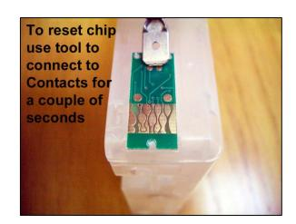
After resetting the chip and re-installing the cartridge, the printer display should show the ink level at 100% for the reset cartridge. If not, remove the cartridge and try resetting the chip again. Chips can be reset to full using this method at any time, so even a cartridge that is still showing 75% full, for example, can be refilled and reset prior to a long print run if required.
