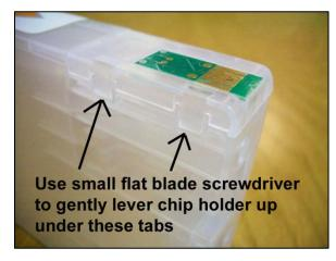
To install the new chip, simply line up the chip holder assembly over the recess in the cartridge and push down on the side of the plastic to snap the new assembly into place. Try to avoid touching the gold contacts on the chip during this operation. After a chip has been changed, it is wise to purchase a new spare chip from your supplier.
