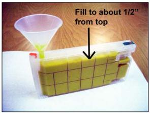
Remove the funnel from the cartridge and insert the rubber bung firmly back into the filling hole. Clean the funnel using water under a faucet, and store in a clean place ready for when the cartridge needs refilling again. Repeat the filling process with each cartridge that you intend to install at this point using a clean funnel for each cartridge and ensuring you fill the correct color ink into the correct color cartridge.
