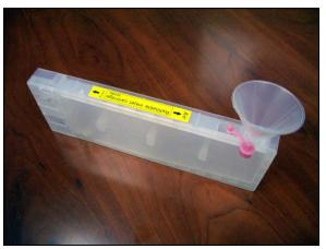
cm) of the top. Remove the funnel and insert the bung back into the filling hole. Wash out the funnel with water under a faucet, dry the funnel with paper towel, and store in a clean, safe place for use the next time you need to refill. Repeat the filling process with each cartridge in turn using a clean funnel for each cartridge and ensuring you fill the correct color ink into the correct color cartridge.
