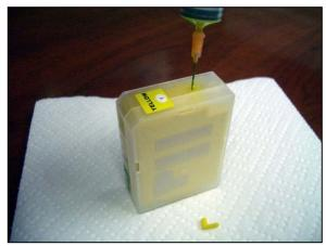
After filling the cartridge, make sure you insert the rubber bung back into the ink fill hole.
