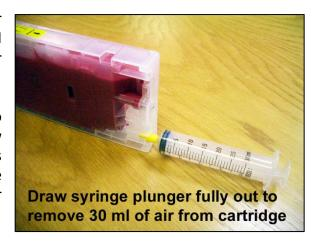
If any ink appears in the syringe during the pressure test, then the cartridge is faulty and should not be installed in a printer. The ink in the cartridge can be saved by pouring it out through the cartridge filling hole. Replacement cartridges are available from the supplier where the kit was purchased.
