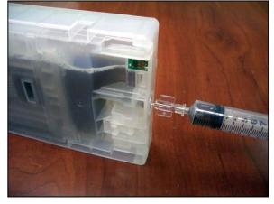
the syringe out with water under a faucet. Repeat this process with each cartridge you intend to install at this point, remembering to wash out the syringe between colors so
