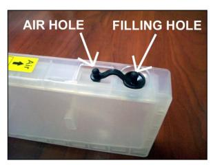
The bigger hole on the top of the cartridge is the ink filling hole and the bung should only be removed from this hole when you are filling a cartridge. The ink filling hole should have the bung pushed in during normal operation.
