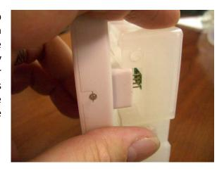
Before refilling, always double check you are putting the correct color ink into the correct color cartridge. To refill a cartridge, simply remove the bung from the filling hole and using a clean funnel, fill the cartridge with ink to within  $\frac{1}{2}$ " (1 cm) of the top surface. Remove the funnel and push the bung back into the filling hole. Wash out the funnel with water under a faucet and keep safe for the next time you need to refill.
